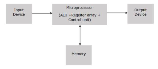
How does a Microprocessor Work?
