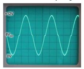
Fig 5.3.5 Crossover Distortion Produced by Fig. 5.3.4
