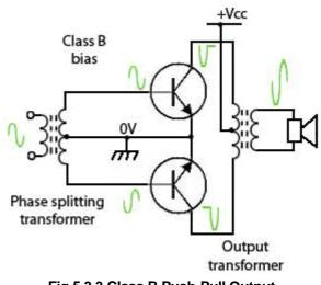
Fig 5.3.3 Class B Push-Pull Output
