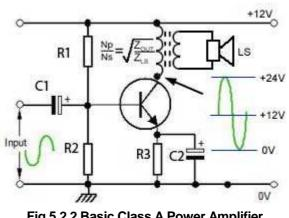
Fig 5.2.2 Basic Class A Power Amplifier
