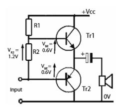
Fig 5.5.2 Applying Class AB Bias
