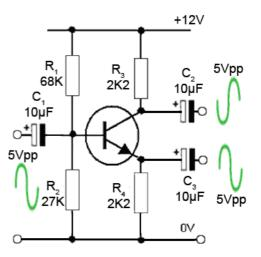
Fig 5.4.2 Phase splitting using a transistor amplifier
