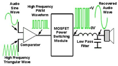
Fig. 5.6.2 Basic Principles of Class D
