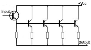
Fig 5.1.5 Power Transistor Connected in Parallel
