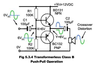
half of  $V_{CC}$  allowing the output to vary between  $V_{CC}$  and 0V. Because the complimentary pair of output transistors (BD131 and BD132 in this case, but any similar pair of output transistors could be used) are working in opposite polarity to each other, the NPN is transistor biased on only during the
