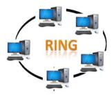
The Ring network is similar to the bus network, the ring network does not rely on a central host computer either. Each computer in the network can communicate directly with any other computer, and each processes its own applications independently. A ring network forms a closed loop and data is sent in one direction only and if a computer in the network fails the data is still able to be transmitted.
