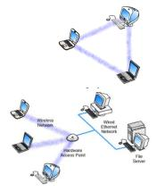
An ad-hoc or peer-to-peer wireless network consists of a number of computers each equipped with a wireless networking interface card. Each computer can communicate directly with all of the other wireless enabled computers.
