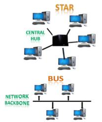
The Star network, a general more simplistic type of topology, has one central hub that connects to three or more computers and the ability to network printers. The major disadvantage is the star network is its vulnerability. All data must pass through one central host computer and if that host fails the entire network will fail.
